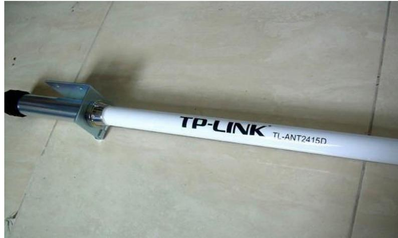
Gambar 2.13 Antena Omnidirectional
