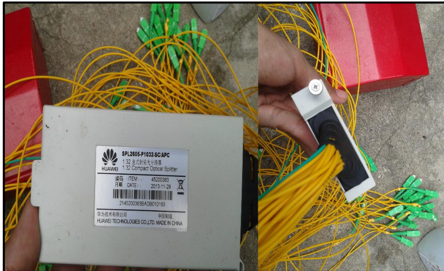
Gambar 3.9 Splitter Huawei SPL2605-P1032 1:32
