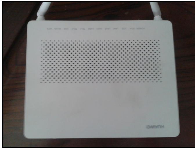
Gambar 3.8 Optical Network Terminal Huawei EchoLife HG8245H
