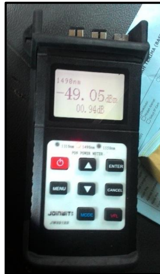
Gambar 3.19 Optical Power Meter JOINWIT JW3212B
