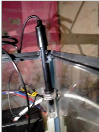
**Gambar 5.22 Tampilan Sensor pH Air**
