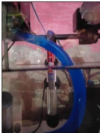
**Gambar 5.36 *Water Heater* Mati Pada Suhu Normal**
