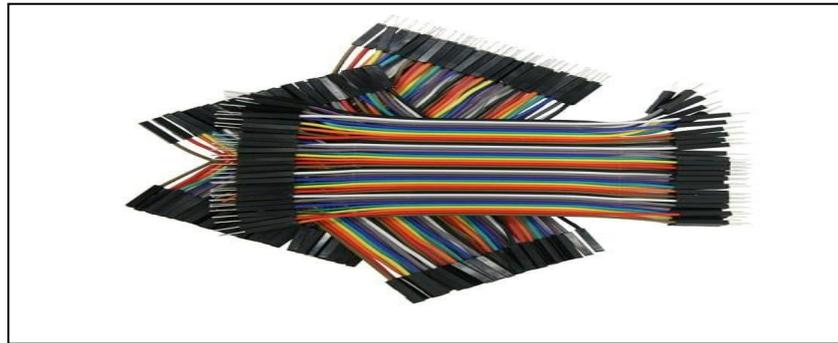
**Gambar 3.2.3 Kabel *Jumper***
