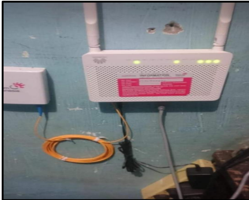
Gambar : 3.2. Access Point Huawei HG8245H
