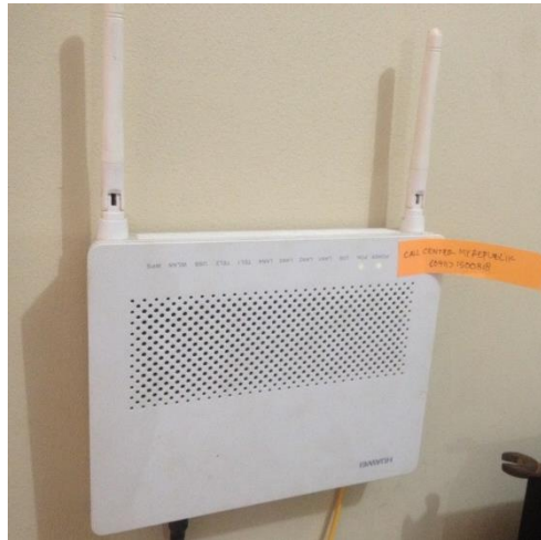
Gambar 3.3 Access Point HUAWEI HG8245A GPON (Sumber PT. Biosron)
